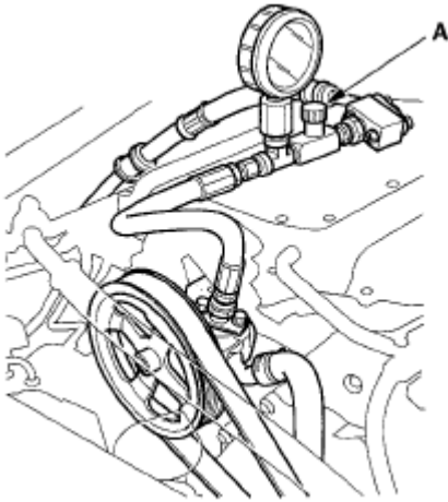
Fig. 11: Identifying Shut-Off Valve Courtesy of AMERICAN HONDA MOTOR CO., INC.
